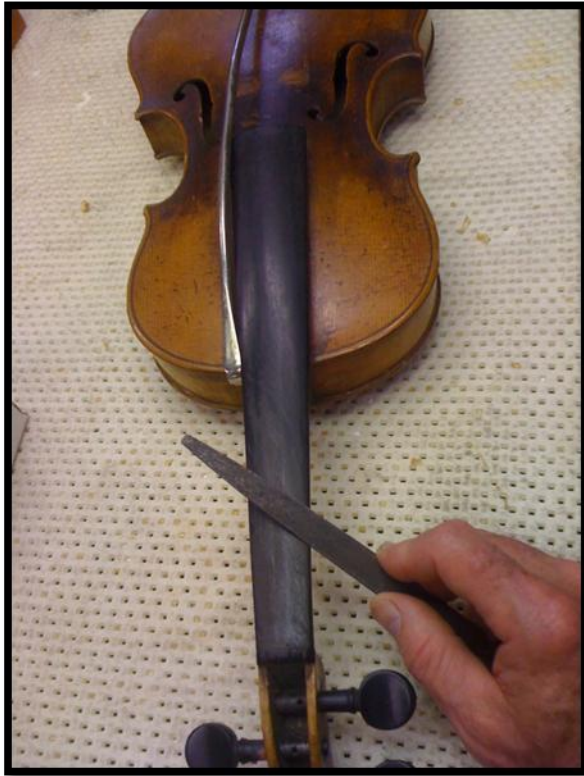
Filing indentations in the fingerboard
